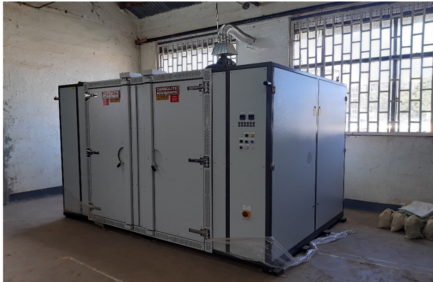
Large sample drying oven after installation
