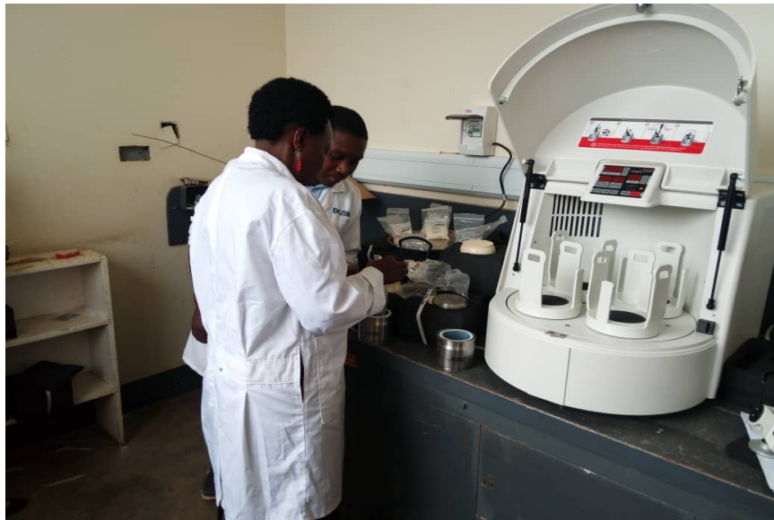
Planetary ball mill during installation
